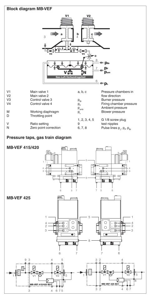
Valve V4 is activated by valve V2. In closed position, valve V4 blocks the chamber under the working diaphragm M from the burner pressure.
